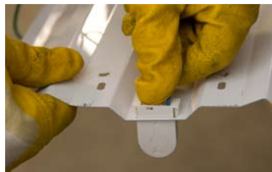
6. Snap in sockets into each end of Reflector Assembly .
